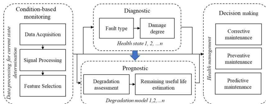
Figure 2 – An overview of condition-based monitoring (CBM)
